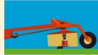
When encountering humps or bumps the mower unit lifts and swings back at the same time
