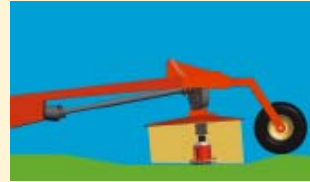
Cutting tight to the ground with Vicon's Free Float Suspension System
