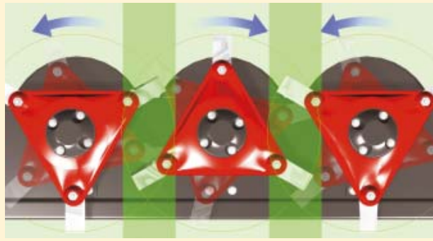
Vicon's contra-rotating three bladed discs provide a wider overlap, ensuring a perfect cut
