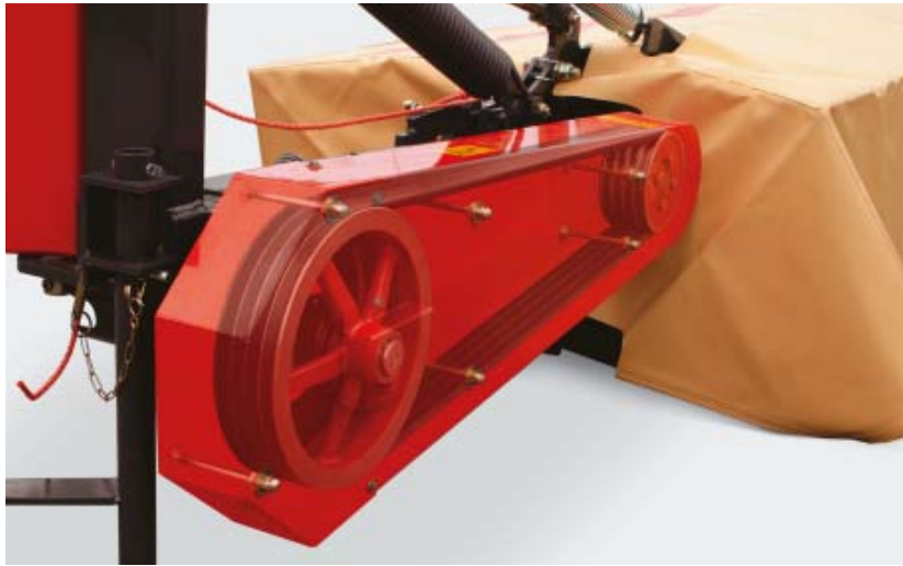
A V-belt drive protects drive line and mower bar in case of foreign obstacles
