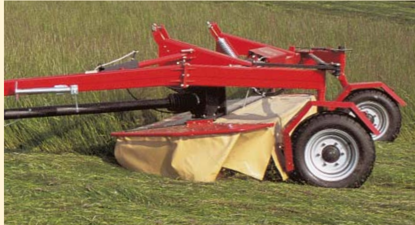
When encountering humps or bumps the mower unit lifts and swings back at the same time
